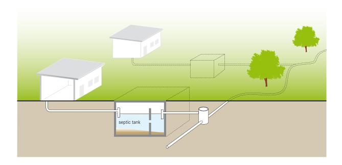
A solids-free sewer is a network of small-diameter pipes that transports pre-treated and solids-free wastewater (such as Septic Tank effluent). It can be installed at a shallow depth and does not require a minimum wastewater flow or slope to function.
